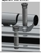
Drill a  $\phi$  11 mm hole in the profile through 3 walls.
