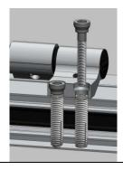
Drill a  $\phi$  11 mm hole in the profile through 3 walls. Insert the TKO and then tighten the wing.
